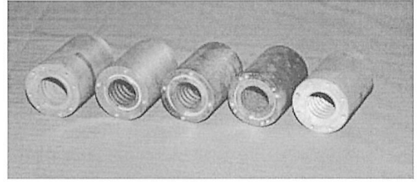
Fig. 3. Photo of five helical groove waveguides.
